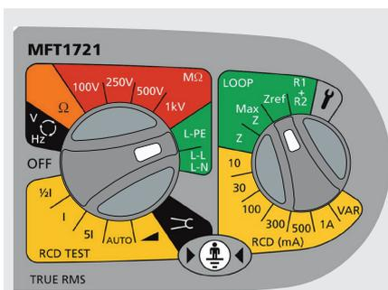
Make a loop measurement using either the Phase to Neutral or Phase to Earth methods above. This value is automatically stored as the reference value. This can be repeated if necessary.
