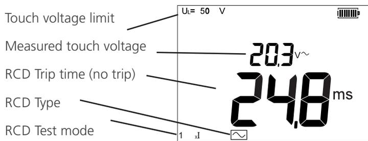
Touch voltage is calculated using the nominal trip current of the RCD x Earth resistance. For example:
