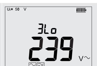
Figure 4. Live Circuit Warning Screen
