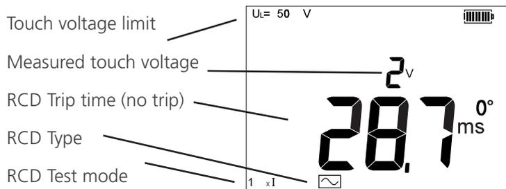
\*any value below 300 ms indicates an RCD has tripped in an adequate time.
