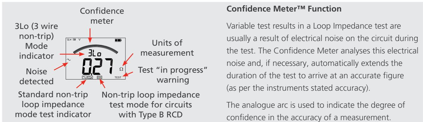
Figure 1. Instrument Display
