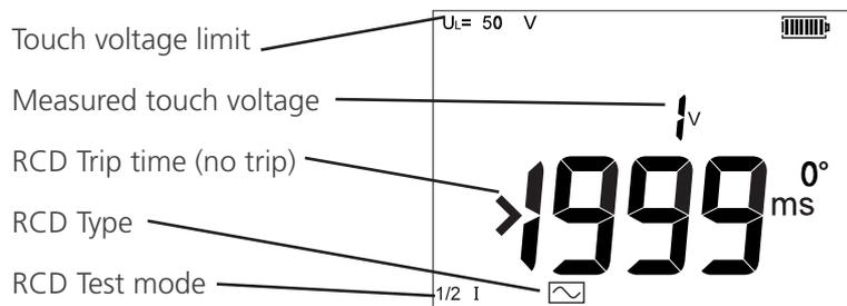
If the RCD Trips, the MFT will flash the “trP” warning and then display the following:
