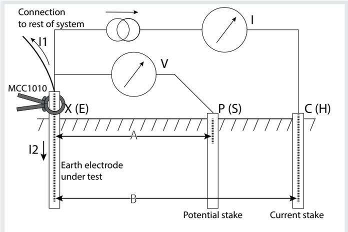
Figure 11: Schematic for three-terminal resistance measurement using
