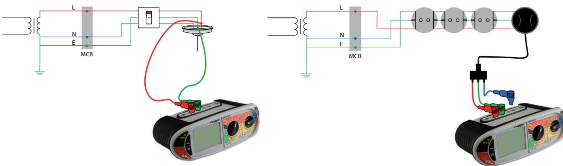
The Blue (L3) test lead can be connected to enable "reverse polarity" warnings
