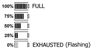
Where NiMH rechargeable batteries are fitted, the battery condition display can be adjusted accordingly. Refer to **"11. Setup options"** on page 52 to change between alkaline and rechargeable batteries.
