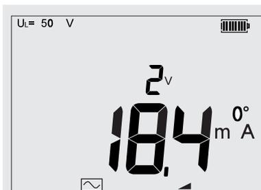
If the RCD fails to trip, >\*\*\*mA is displayed, where \*\*\* = 110% of the nominal RCD trip current.
