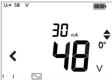
3. Use the UP and DOWN arrows on the right hand TEST and LOCK buttons to set the tripping current to match that on the variable RCD.
