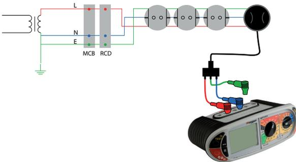
4. Press and release the TEST button to start the test.
