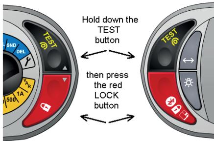
To release the "Locked on" insulation test, press the TEST button.
