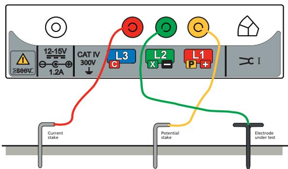
2. Set the rotary selector switch to the **2P** / **3P** position.
