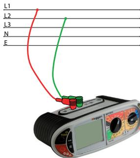
3. To start test, press and hold either of the TEST buttons,
