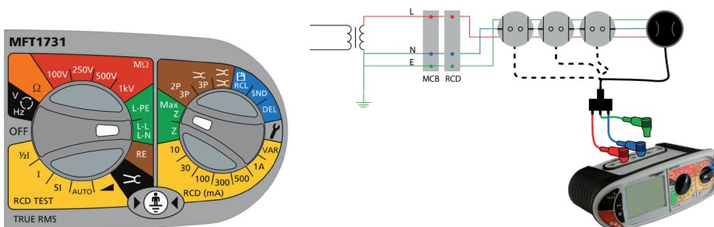
3. Connect the test leads to the Phase (L1) and Earth (L2) or Phase (L1) and Neutral (L3) terminals on the tester depending on the selection of the LEFT rotary range knob.
