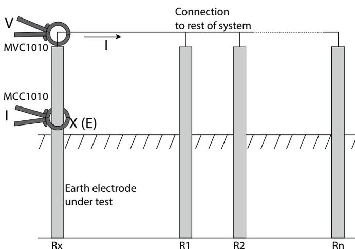
Figure 12: Schematic for two-clamp stake-less resistance measurement
