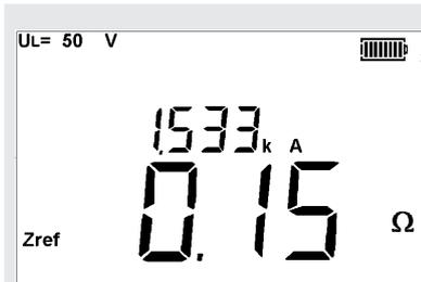
2. Switch the range knob to R1+R2 and make loop impedance tests as previously.
