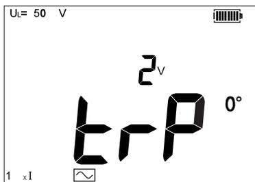
**NOTE :** For Type AC RCDs there is no need to perform a 180° test on the 1/2I mode, as the test uses a full AC waveform.
