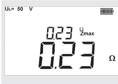
6. Move to the 2nd socket to be tested and make another loop test. If the result is less than the first the large readout will show the new value but the small readout will remain unchanged. If the new value is higher, the small readout will be updated accordingly, as below:
