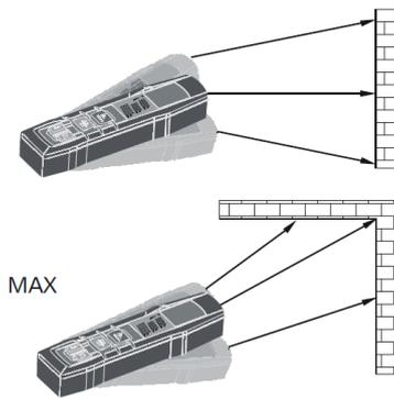
The continuous measurement updates the measured value continuously in the third (summary) line of the display. The corresponding minimum and maximum values are displayed dynamically in the first and second lines respectively, updated every 0.5 seconds.
