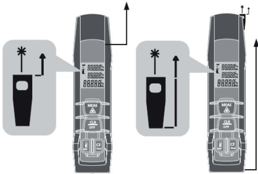
The default measurement reference is taken from the rear of the instrument. Long press this button prior to taking a measurement to switch between the front and rear edge. A special beep sounds whenever the reference setting is changed. When powering up the meter, the measurement reference automatically returns to the default setting (rear reference).
