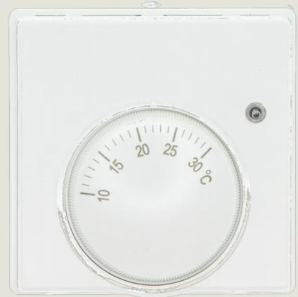
Designed for wall mounting, with 60mm fixing centres for back-box compatibility, and suitable for in-wall or surface-run wiring connection. The thermostat cover incorporates four breakouts for surface-run conduit. The temperature regulation mechanism is the well-proven sealed bellows system.
